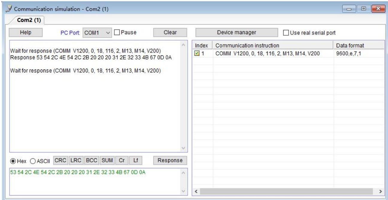
Click on the "simulation", open the communication simulation in the debug menu, fill in the data in the answering area, click on the "answer" to simulate the communication program, if the serial interface of computer is actually connected to instrumentation, you can check the "use the actual serial port" so that the software can co-simulation with the actual instrument, very convenient. The final simulation program is as follows:
