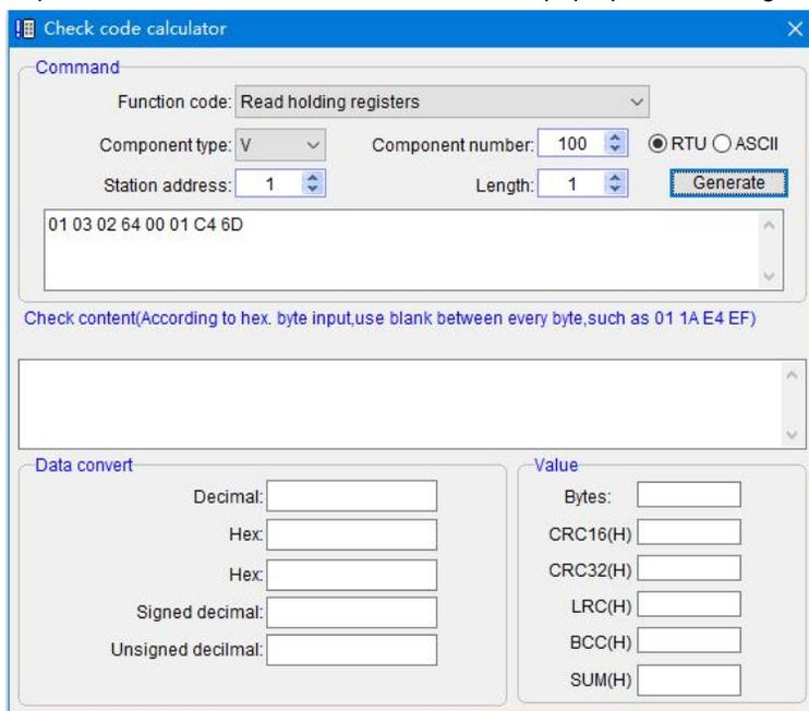
We choose the function code, set the type of components, component number, station number of slave PLC and so on, then click generate, you can get the command: 01 03 02 64 00 01 C4 6D, the command which sent by master can help to read the V100 value of PLC .
