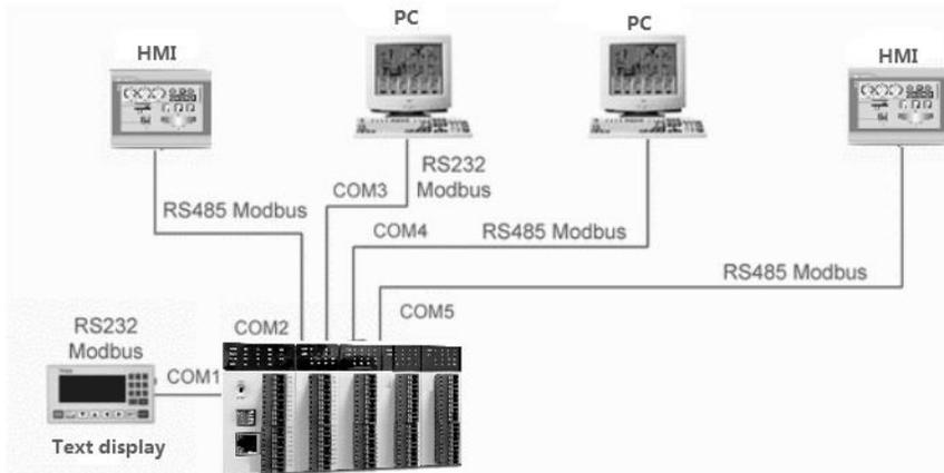
There is no need to write any program when PLC is used as slave, the default parameter is 19200 N 8 2 RTU, station number is 1. For configuration software and touch screen, which has the built-in HNC driver can directly select HNC driver, if there is no HNC driver, you can choose Modicon's Modbus driver. The corresponding Modbus communication code table of HNC is as the following figure:
