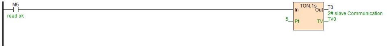
Communication disconnection time can be set according to the actual, the above when M5 is more than 5 seconds in OFF state, T0 coil will indicates communication disconnection alarm.
