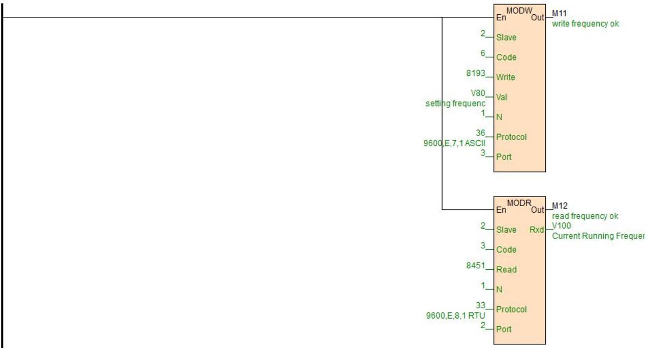
Port = 3, in this example, it indicates the communication port of AE-1C. 8193 can be quickly entered, such as put the mouse on the "Write" terminal, then it can directly enter 0x2001.
