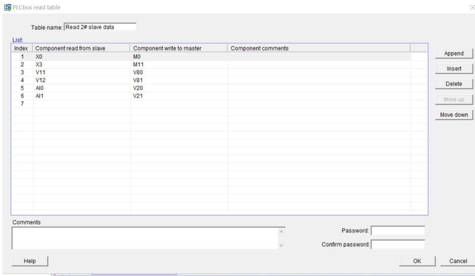
In the HNC PLC programming software, set up PLCbus write communication table, as follows:
